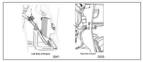
Figure 4-21 Fuel Shut Off Valves
